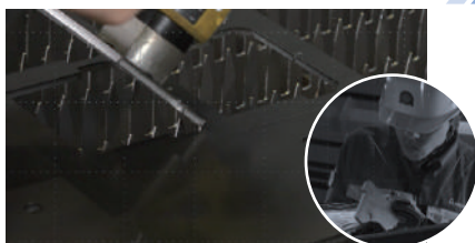
Secondary process required to remove joint marks
