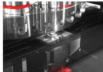
Only the die required for processing is raised and lowered.
