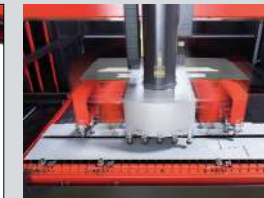
Rotation and extension/contraction of the suction cup unit to accommodate various products
