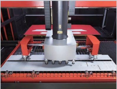
Rotation and extension/contraction of the suction cup unit to accommodate various products
