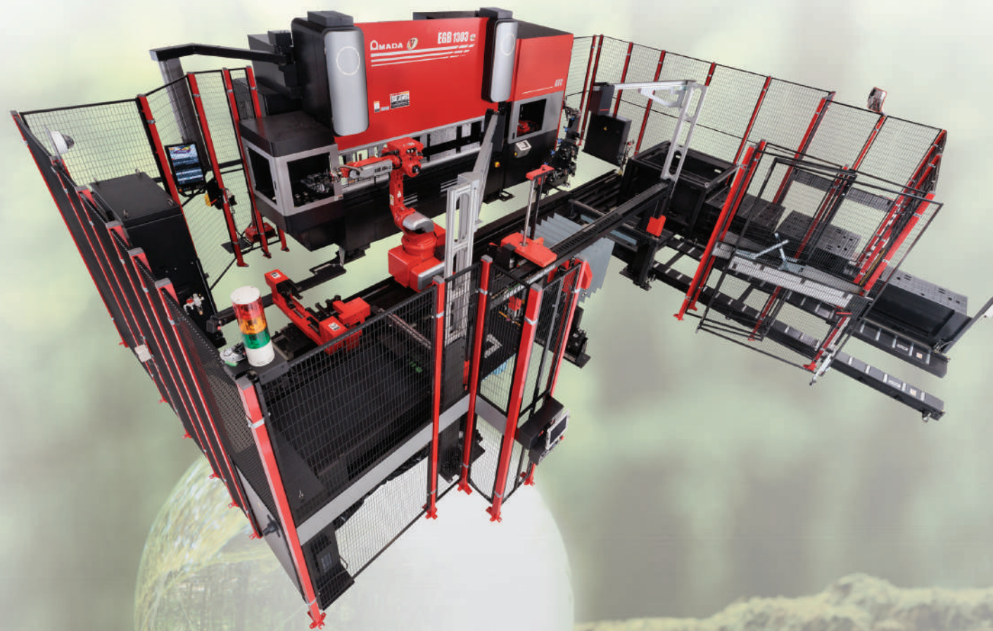
General-purpose Automatic Bending System with Electric Servo Drive
