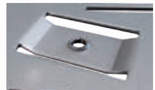
Downward bridge forming
